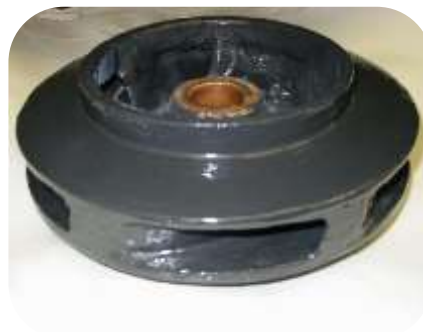
Impeller from a sea water pump was badly eroded. The pump was obsolete and no spare parts were available. The surface of the impeller was rebuilt using 301 Epoxy Resin with glass fillers and then machined to a smooth finish. Once cured 2 coats of 202 Ceramic Repair Fluid were applied to complete the repair
