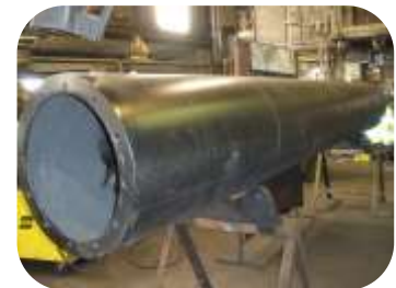
Process vessel required rebuilding and resurfacing. Internal substrates were mechanically abraded and relined using 202 Ceramic Repair Fluid
